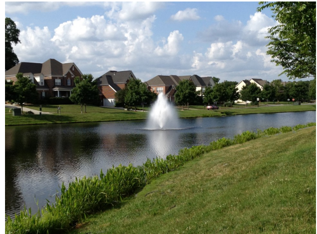
Floating fountain aerators provide effective oxygenation in shallow lakes and ponds, which can help reduce undesirable algae by facilitating the conversion of phosphorus to forms that do not sustain algae growth.
