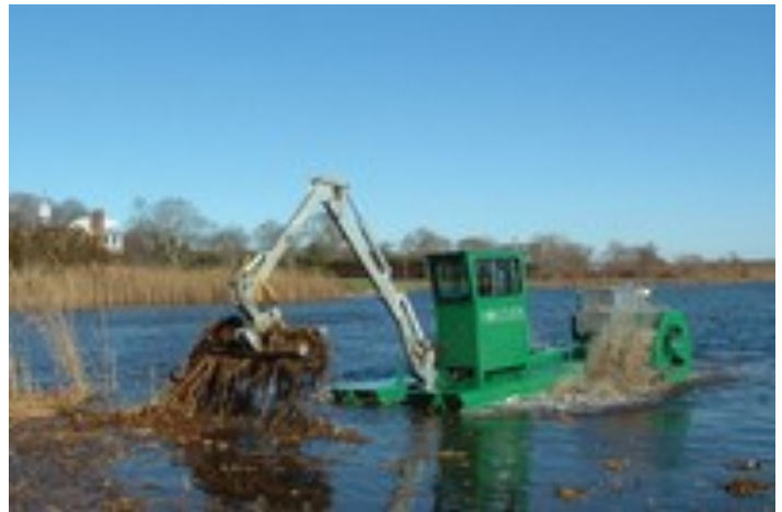
Hydro-raking can be a less invasive and more cost efficient alternate to traditional dredging, which is often times one of the most expensive projects a community will ever face.
